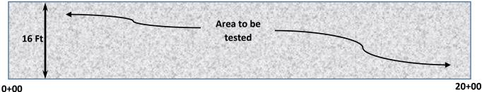
Due to a width of 16 feet, each test section must not exceed 1,500 feet. Therefore, a minimum of two test sections are needed to represent the area in this example. In this case, best practice procedures would involve dividing the 2,000 foot area into two 1,000 foot test sections. Web-link provided below to the *Nuclear Density Testing Manual*:
